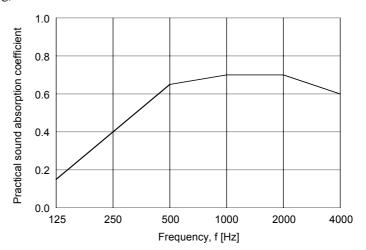
Practical sound absorption coefficient, weighted sound absorption coefficient, and absorption class according to EN ISO 11654:1997:
